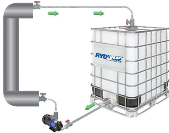
Circulation set up for cleaning pipeline with RYDLYME . Visit our website for available pumping systems!
