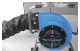
Detail of the quick installation system of the hoses on the tool mouth
