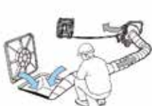
Aspiration in manholes and closed ambients
