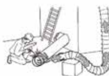
Suction of welding fumes in indoor works
