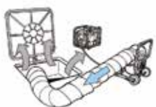
Ventilation of manholes and closed ambients
