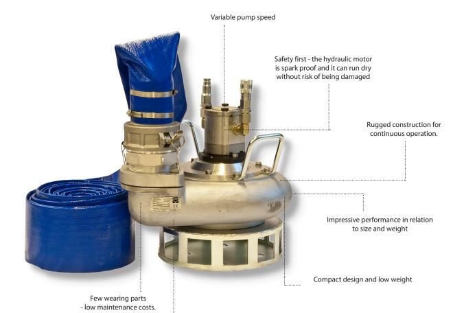
Pumps every tasks - pumps in clean water, contaminated water and slurry.
