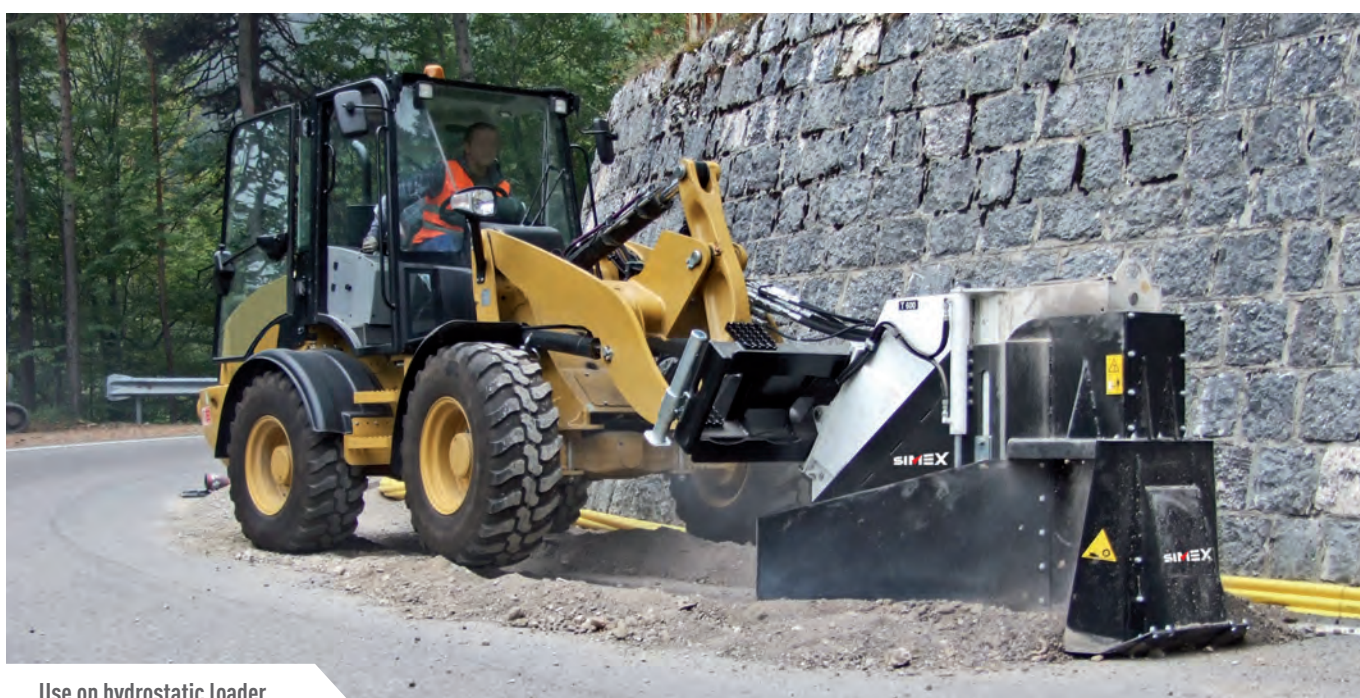
Aspiration of milled material
